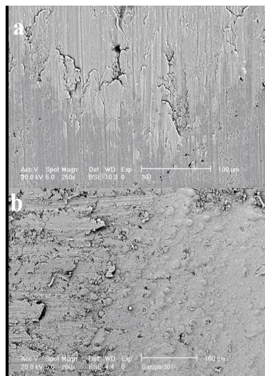
Fig. 10. SEM micrographs of surface of coated sample following abrasive wear with 355-425 \mu\text{m} silica-steel wheel as a function of environment: (a) dry-plan view (b) wet-plan view
